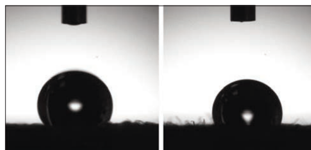
Fig. 8. Water contact angle results of PP and PP+PDA fabrics
